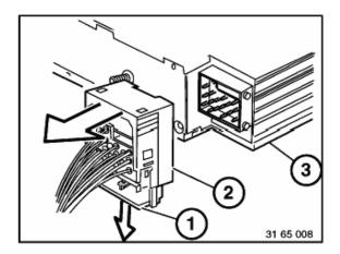
Remove retaining bracket (1) and remove connector (2) from radio (3).
