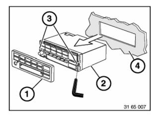
Remove finisher (1), unfasten left or right screws (3) and remove radio (2) through radio aperture.
